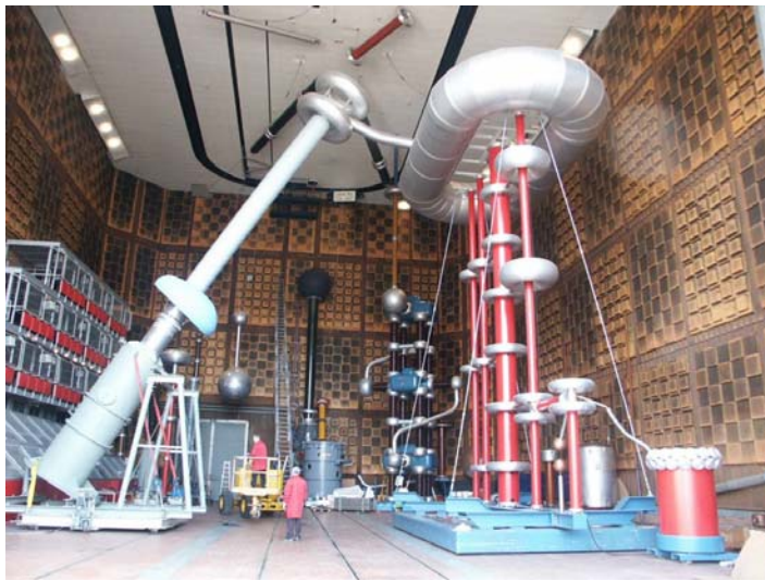
Fig. 19 DC test of an 800 kV transformer bushing
