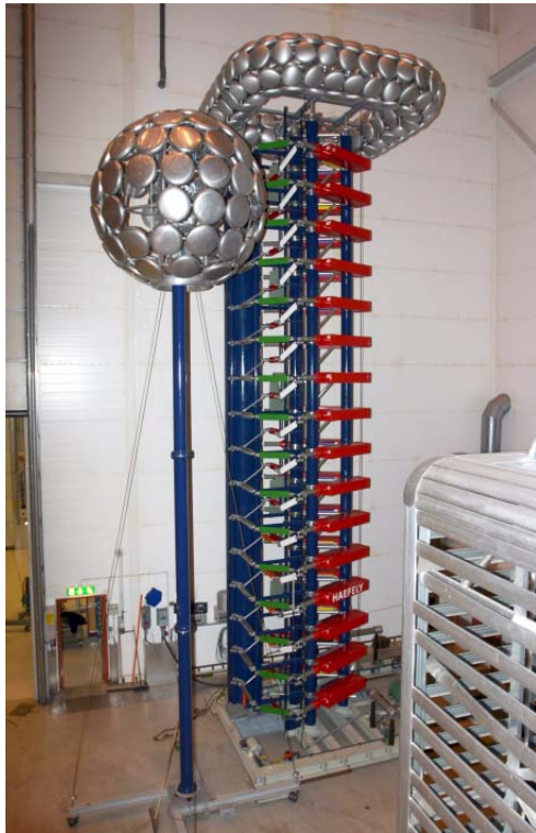
Fig. 13: Impulse generator, 16 stages, maximum charging voltage 3200 kV, energy 240 kJ (Manufacturer: Haefely AG, Basel, Switzerland)
