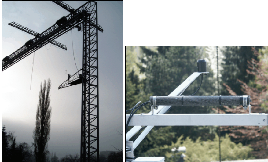
Fig. 3: Weather station at the test laboratory in Graz with the conductor model
