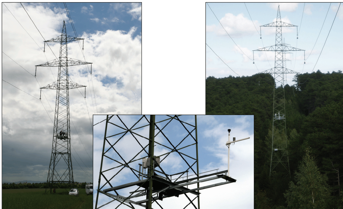
Fig. 2: Weather stations at the 220 kV transmission line (left: position flat country, right: position hill sided in the forest, middle: weather station platform)
