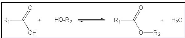
Figure 2. Example of ester synthesis: Synthesis of carbon acid ester: Left Side: acid and alcohol, react onto Ester and Water on the right side [4]
