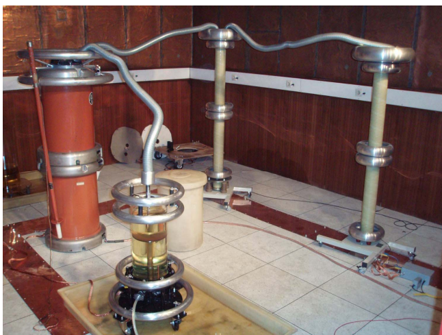
Figure 5. Test arrangement for the partial discharge measurement
