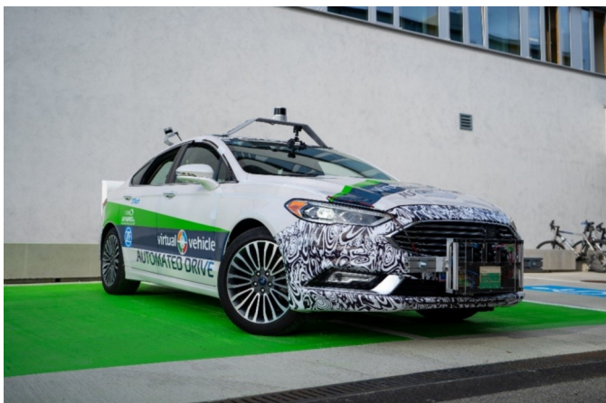
Fig. 6. Research vehicle that has mounted the Sensors Fusion Platform in the front.
