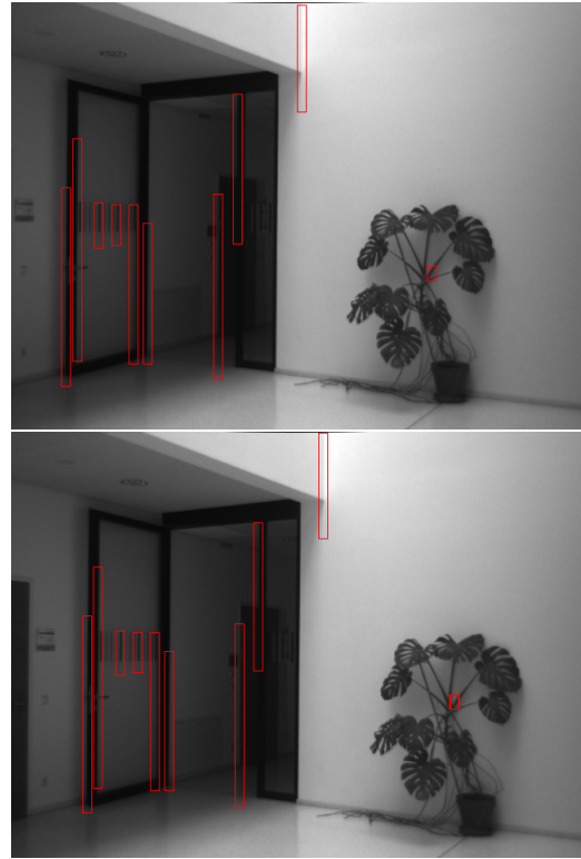
Figure 4: Direct image alignment using patches around lines. Left: Keyframe, where lines are detected and patches around lines (red boxes) are extracted. Right: Image to align. Red boxes are shifted according to the proposed new pose until a minimal photometric error is reached.
