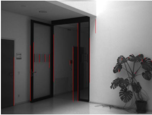
Figure 3: Vertical lines detected with our line detection algorithm. One can see that the lines are not detected over the whole length all the time. This is due to slight gravity misalignment of the images or due to changing light conditions.
