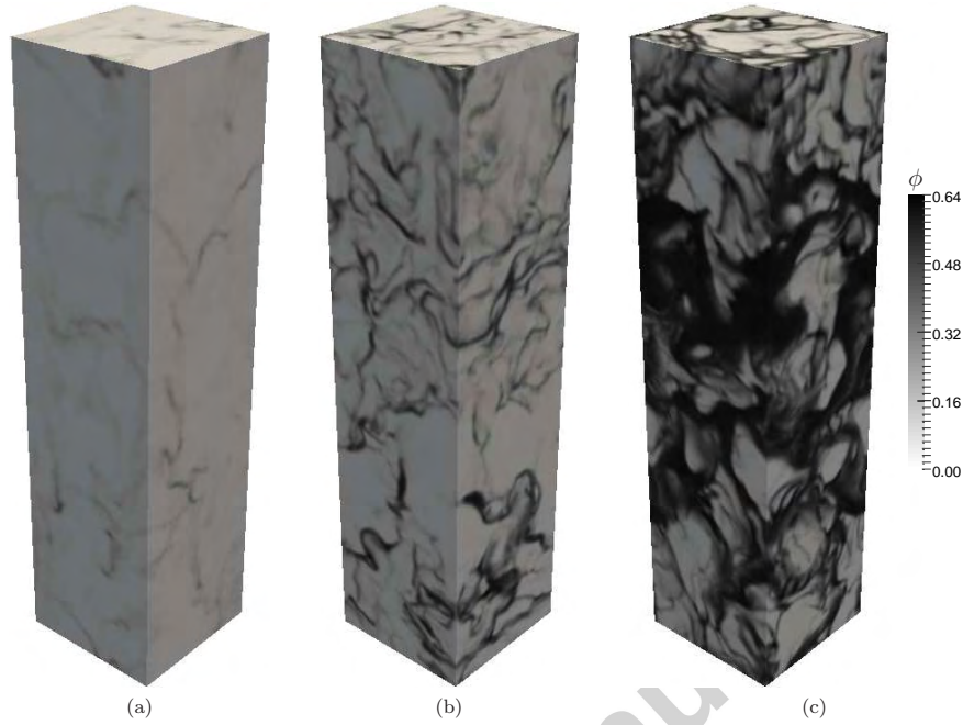
Figure 2: Snapshots of the particle volume fraction field in a periodic domain. Simulations' parameters are listed in Table 1. Domain-averaged particle volume fraction \langle \phi \rangle is (a) 0.02, (b) 0.1 and (c) 0.3. The gray scale axis ranges from 0 (white) to 0.64 (black). Particle Froude number is 88.4.
