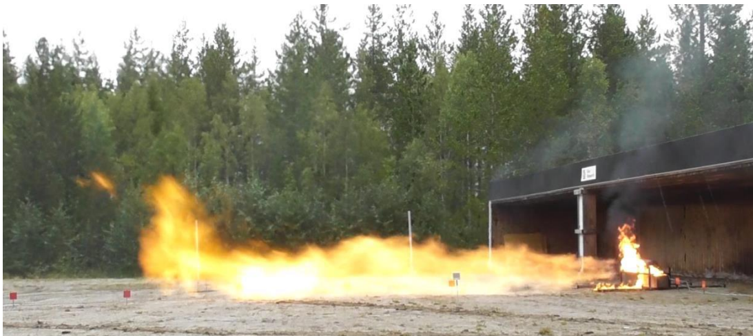
Figure 3: Test of a gas container under fire condition [7]
