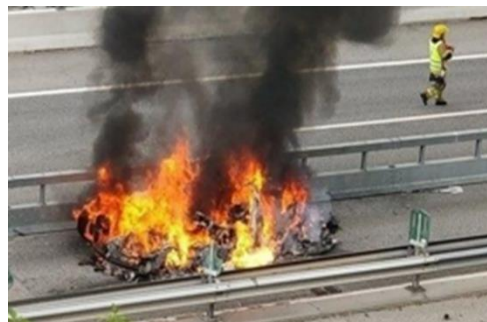
Figure 7 BEV on fire after the car hit the guard rail [33]
