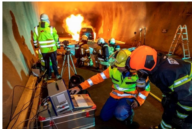
Figure 4: Full scale fire test of a BEV [10] © TUG/Lunghammer
