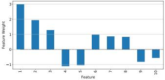
Fig. 3: Model features ranked by their respective contributions (Features: 1 = 'cwt\_coeff\_widths\_(2,5,10,20)\_coeff\_9\_w\_2', 2 = 'quantile\_q\_0.9', 3 = 'mean\_second\_derivative\_central', 4 = 'fft\_coeff\_4\_attr\_real', 5 = 'fft\_coeff\_3\_attr\_real', 6 = 'minimum', 7 = 'fft\_coeff\_2\_attr\_imag', 8 = 'quantile\_q\_0.4', 9 = 'fft\_coeff\_5\_attr\_real', 10 = 'f\_agg\_mean\_isAbs\_true')
