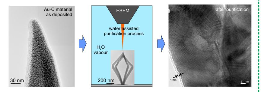
By changing the purification from 2-dimensional to freestanding 3-dimensional structures, the process parameter (electron dose, purification current, dwell time,...) have to be adapted slightly. The purified structures are
