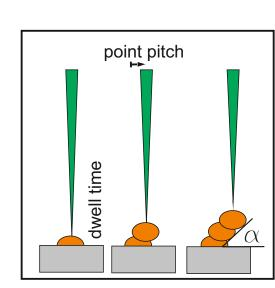
Simple freestanding 3-dimensional nanostructures can be fabricated with FEBID in one single step by using suitable pulse durations (dwell times, DT) and pixel distances (point pitch, PoP).
