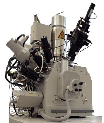
Focused Electron Beam Induced Deposition (FEBID) uses the highly localized decomposition of surface adsorbed precursor molecules via electrons to fabricate functional nanostructures.
