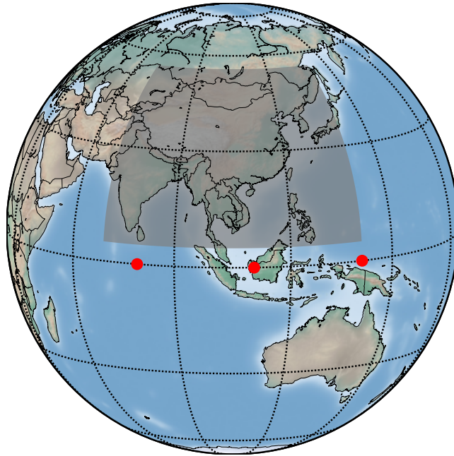
Fig. 2.1: The BDS-1 service area from longitude 70°E to 140°E and from latitude 5°N, as defined by Yang et al. (2017b). The red dots indicate the location of the GEO satellites.
