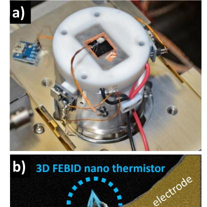
This temperature rise results in a reduced residence times of the precursor and therefore to lower growth rates<sup>[2]</sup> and consequently to stability problems for larger 3D structures. Based on those insights, we here turn around the situation and lower the substrate temperature with a home-build Peltier cooling stage (Fig. 2a) to study the implications on growth stability and fabrication precision in *3D*-FEBID in a temperature
