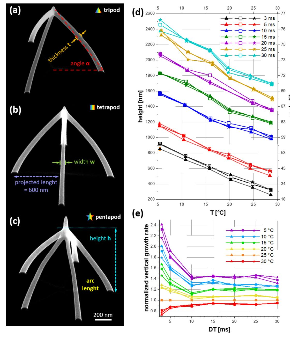
The SEM based growth analysis of tri-, tetra- and pentapods (Fig. 3a-c), fabricated from MeCpPt<sup>(IV)</sup>Me<sub>3</sub> at substrate temperatures T of 5, 10, 15, 20, 25 and 30 °C revealed
