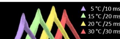
Figure 5: Pillar growth rates after the merging zone, demonstrating that for proper 3D-FEBID design the support geometry has to be considered.<sup>[3]</sup>
