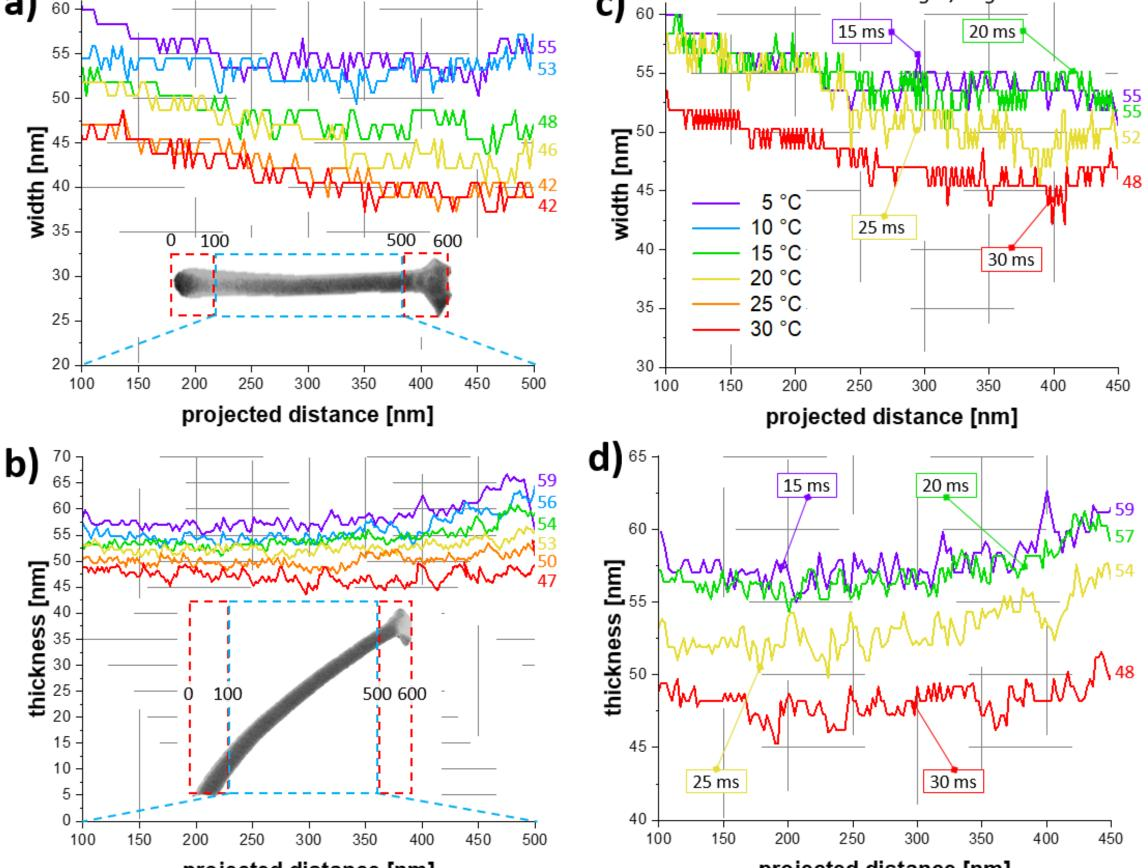
a function of the projected length showed slightly larger wires at reduced substrate temperatures. This is valid for both, wires fabricated under constant DTs of 15 ms (Fig. 4a; Fig. 4b), as well as for constant heights (Fig. 4c; Fig 4d).
