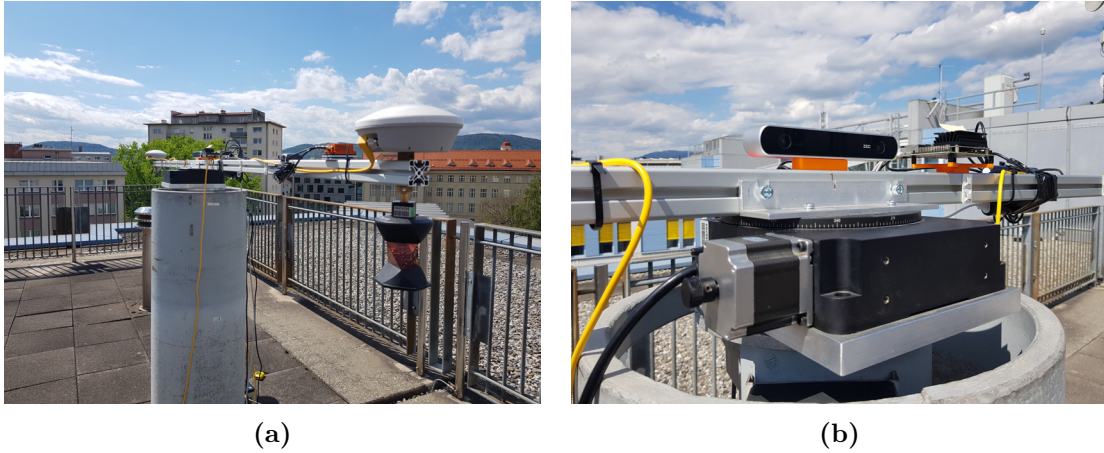
Figure 6.13: Sensor evaluation setup on a pillar with known coordinates. (a) A 360°-prism was mounted below the GNSS antenna for reference tracking. (b) A motorized rotation stage rotates the aluminium profile on which the sensors are mounted.
