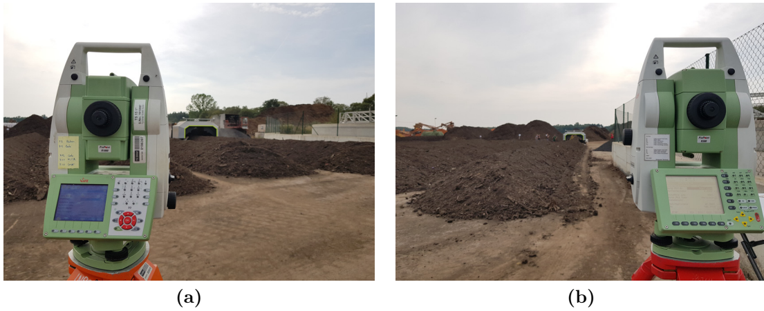
Figure 8.9: Tracking the reference trajectory with (a) a Leica TS15, and (b) a Leica TCRA1201.
