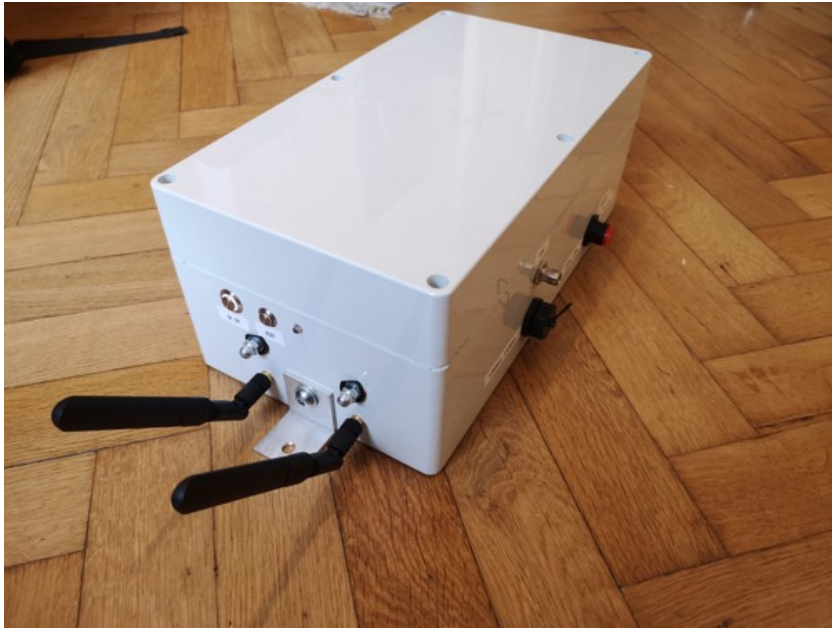
Figure 8.5: Picture of the box protecting the Jetson Nano computing unit and the GNSS receiver from dust and dirt.
