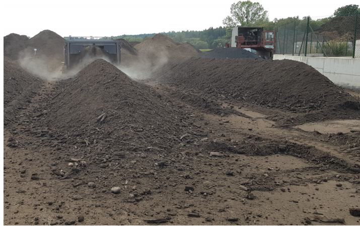
Figure 9.14: Picture of the first windrow (on the right side) after being turned by the automatically steered compost turner, and the second windrow (on the left side) while being turned.
