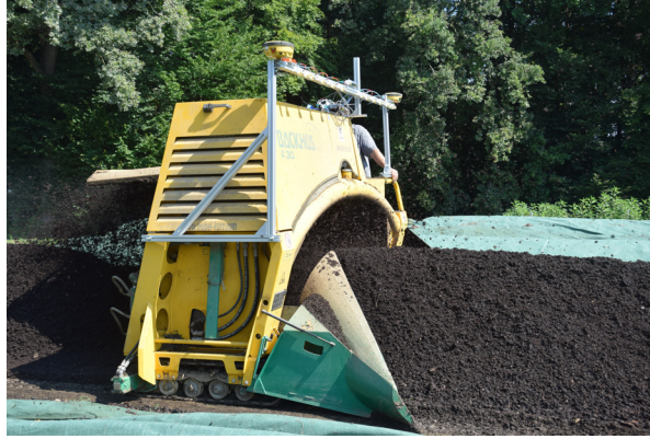
Figure 6.4: Picture of the Backhus A30 used in the pre-study. The navigation sensors are mounted on an aluminium profile.
