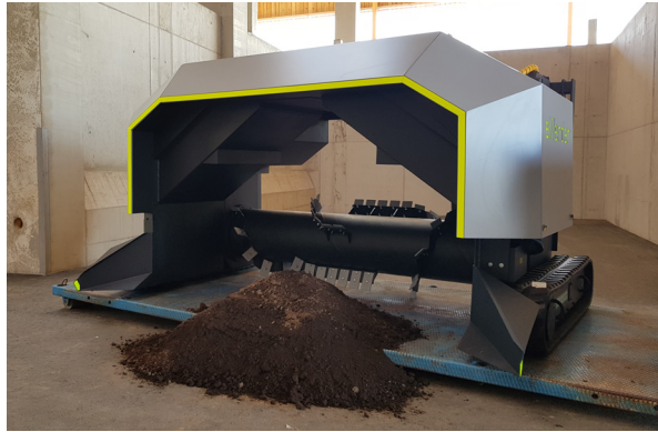
Figure 6.3: Picture of the prototype of the electrically driven, self-driving compost turner.
