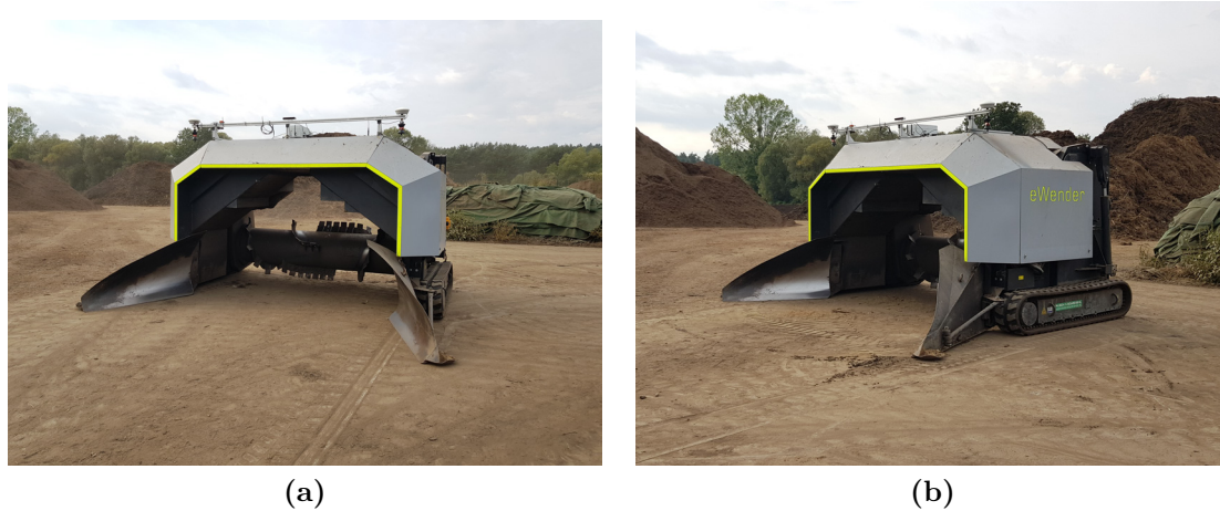
Figure 8.8: eWender e35eco equipped with the navigation sensors for the automatic steering system (a) seen from the front, (b) seen from the side.
