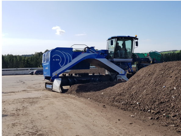
Figure 1.2: A compost turner (Backhus A55) at a composting site in Alberndorf in der Riedmark, Austria. The organic material is turned with the machine’s spiked drum.
