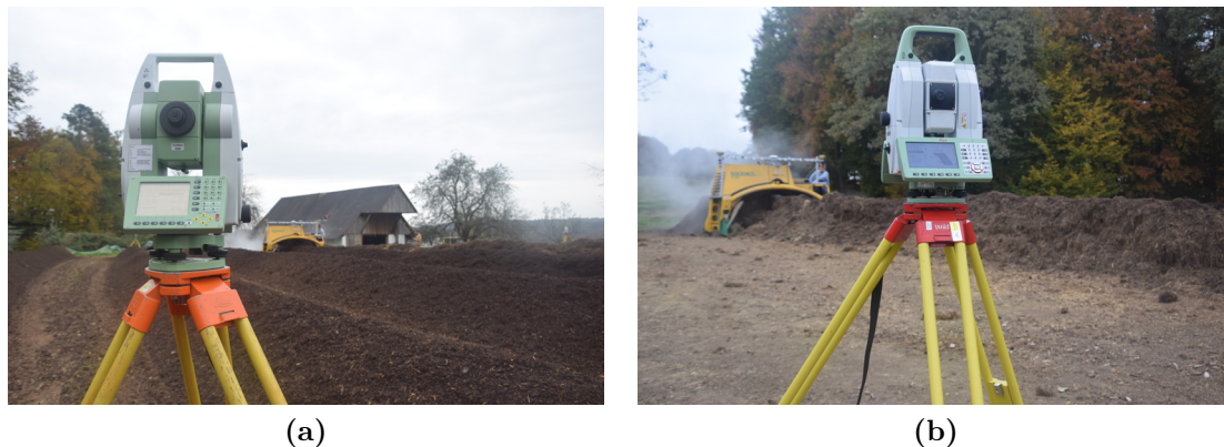
Figure 6.6: The reference trajectory was obtained by tracking two 360^\circ prisms mounted on the compost turner with two robotic total stations: (a) a Leica TCRA1201, and (b) a Leica Nova MS60.
