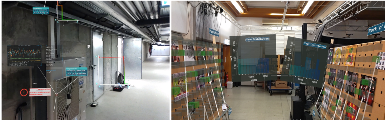
Fig. 1. Example application built with RagRug: (left) Hot air emissions in the basement. All measurements are taken in real-time by stationary sensors observing heat distribution. Multiple sensors are visually annotated with panels giving detailed sensor characteristics, including two types of time-series plots of temperature. (right) An application supporting the design of an exhibition of musical artefacts. Each of the two exhibition walls on the left and right hand side has been decorated with multiple exhibits. For each decorated position, a leader line extends to a timeline shown at the bottom of the wall.
