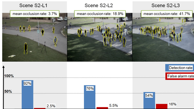
Fig. 3. Top row: Sample detection results and mean occlusion rates (latter computed from annotations) obtained for the PETS2009 dataset [28]. Bottom row: Obtained detection and false alarm rates computed from all frames when using our framework.
