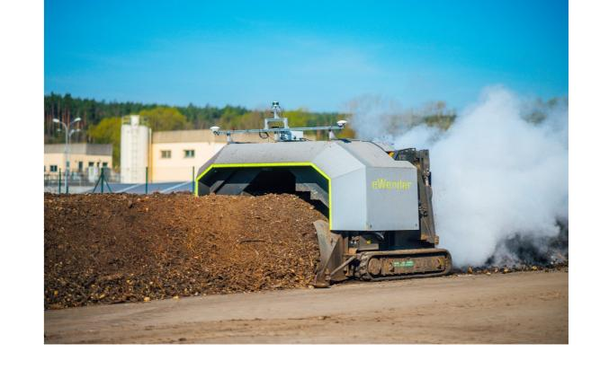
Demonstration with a prototype autonomous compost turner within an industrial setting: Showcasing the successful interaction of the IIoT module, the navigation module, the sensor technology and the drive train.
