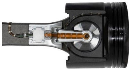
Figure 1: Piston instrumented with a telemetry system
