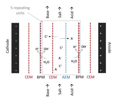
Figure 1. Schematic of membrane configuration and separation mode in the EDBM membrane stack.
