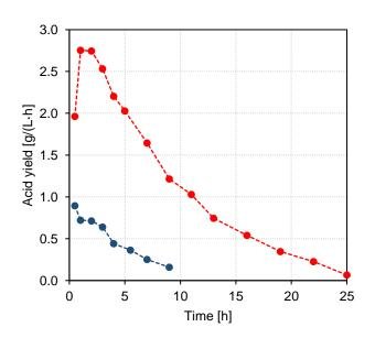
**Figure 7.** Yields of total acids in the acid compartment for the EDBM experiment with BL permeate (•) and BL model solution (•).
