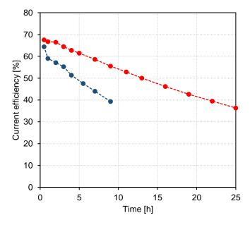
**Figure 6.** Current efficiency development during the EDBM experiment with BL permeate (•) and BL model solution (•).
