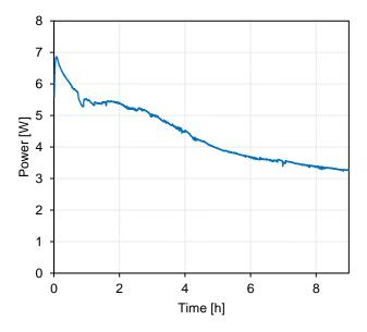
**Figure 2.** Power over treatment time for the batch EDBM treatment of BL permeate,  $U_{cell} = 10 V$  (constant).
