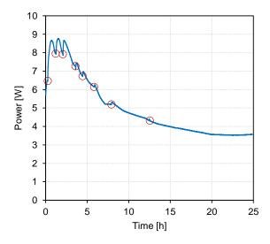
**Figure 4.** Power over treatment time for the batch EDBM treatment of BL model solution,  $U_{cell} = 10 V$  (constant). The red circles mark the points of NaOH addition.
