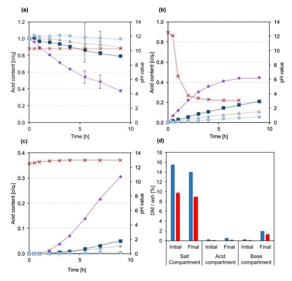
**Figure 3.** Development of carboxylic acid concentrations and pH value over the course of the EDBM experiment with BL permeate. (a) Salt compartment; (b) acid compartment; (c) base compartment. For (**a**–**c**): ■ glycolic acid, • lactic acid, ◆ formic acid, ▲ acetic acid, X pH value. (d) DM (■) and ash (■) content measured in the initial and final samples from the three compartments.
