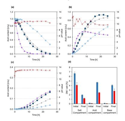
**Figure 5.** Development of carboxylic acid concentrations and pH value over the course of the longterm EDBM experiment with BL model solution. (a) Salt compartment; (b) acid compartment; (c) base compartment. For (**a**–**c**): ■ glycolic acid, ● lactic acid, ◆ formic acid, ▲ acetic acid, **X** pH value. (d) DM (■) and ash (■) content measured in the initial and final samples from the three compartments.
