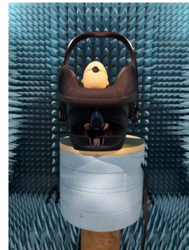
(b) Mounted baby dummy on the table at zero degree azimuth.
