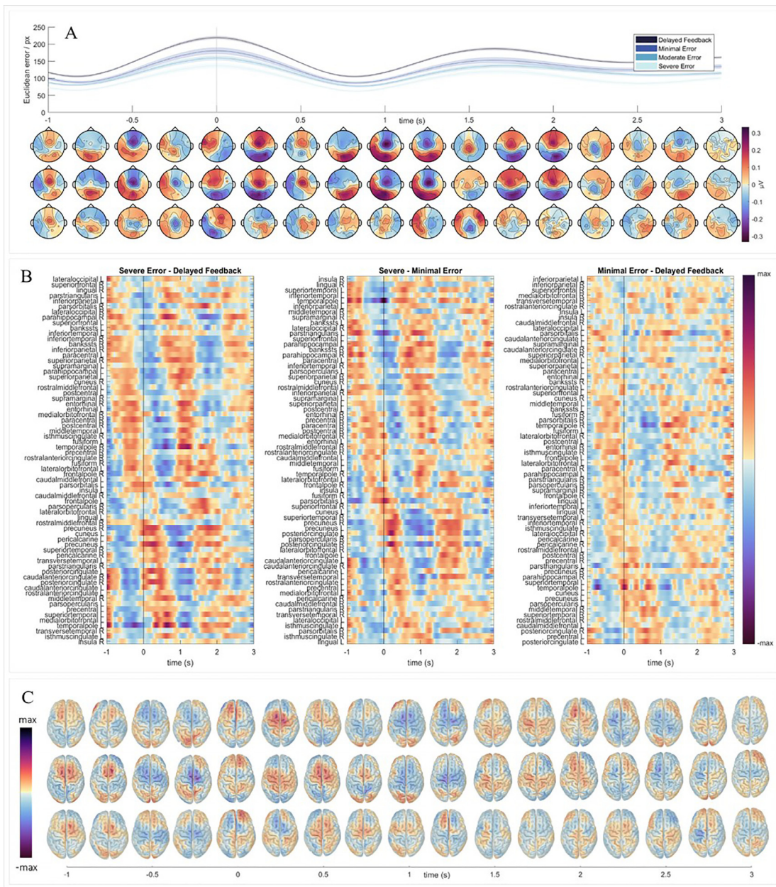
Fig. 7. Dataset 2. A (top) Grand average Euclidean error signal between target (snake) and feedback (assistive robotic arm) for the four feedback conditions Delayed Feedback, Minimal Error, Moderate Error, and Severe Error. (bottom) Grand average difference patterns in EEG signals, time-locked to local maxima of the Euclidean error signal ( t = 0 ms) for Severe-Minimal Error, Severe Error-Delayed Feedback and Minimal Error-Delayed Feedback feedback conditions (topographical maps, top down). B Grand average difference in the scout signals for Severe-Minimal Error, Severe Error-Delayed Feedback and Minimal Error-Delayed Feedback conditions (left to right). C Grand average full cortical difference maps for Severe-Minimal Error, Severe Error-Delayed Feedback, and Minimal Error-Delayed Feedback conditions (top down). All depicted results correspond to findings in the delta frequency band.
