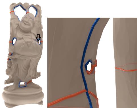
Figure 16: The Happy Buddha model (left) and a zoom-in on the area marked by the arrow showing the effect of a tiny handle spanned by only three triangles on the output of our variational method.
