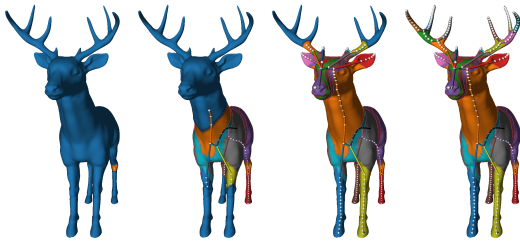
Figure 11: Reeb graph creation on the genus-0 Deer model. Please note how the branching structure of the deer horns is well captured.
