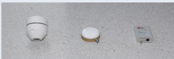
Fig. 4: Evaluated low cost GNSS equipment FLTR: AT575-142 (300 €), Antcom G3 (420 €), ublox LEA6T (300 €)
