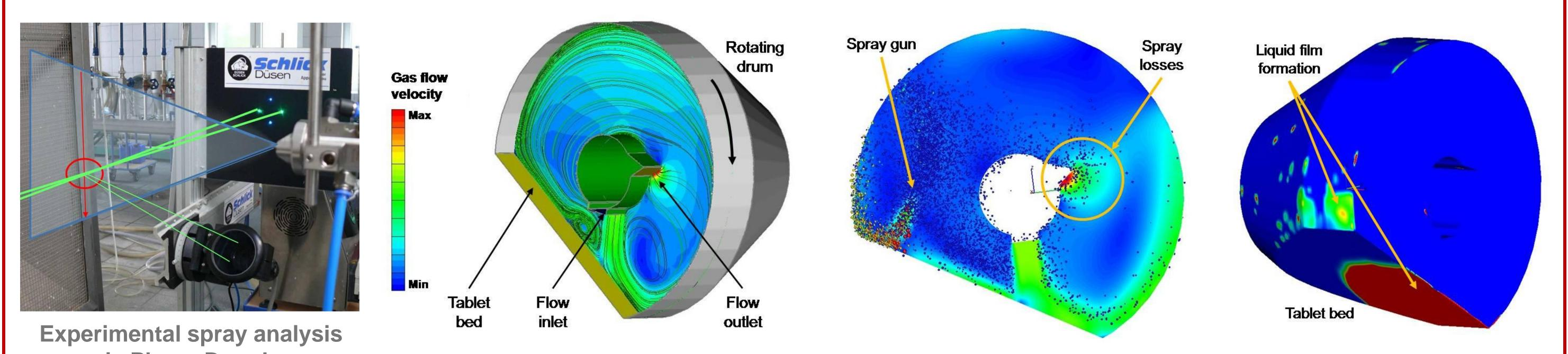
via Phase-Doppler Anemometry (PDA) system
