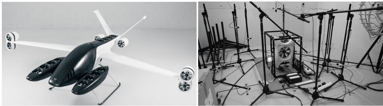
Figure 2. The device under test during the measurement campaign ( right ) is one fan of the propulsion assemblies, which are arranged left and right of the fuselage of the APELEON X1 ( left ).
