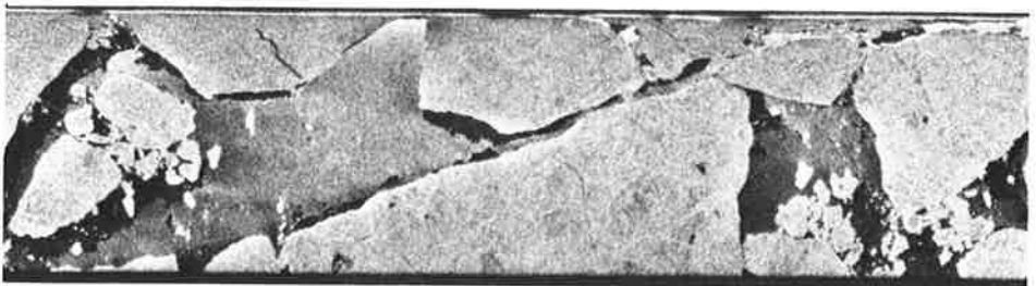
Fig. 1. Side-looking radar image of Arctic sea ice. Arctic ice floes imaged on 18 August 1976 by JPL's L-band synthetic aperture radar system; images were taken during a mission for the Arctic Ice Dynamics Joint Experiment (AIDJEX). Scale: 3 km
