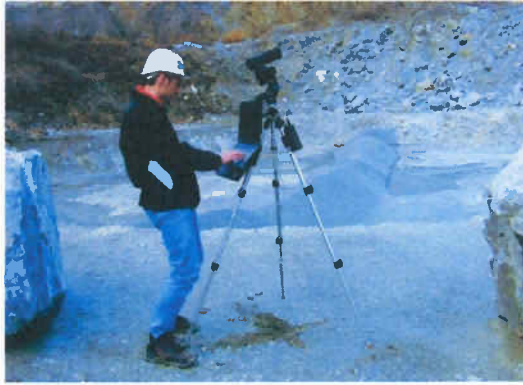
Fig. 1 Rotating CCD line-scan camera mounted on a tripod for imaging with flexible base width.
