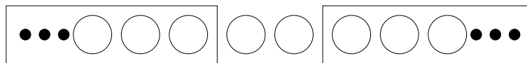
Figure 1.13: The DMRG method. There is a system block to the right and an environment block to the left. The two sites in the center are added at a particular step.
