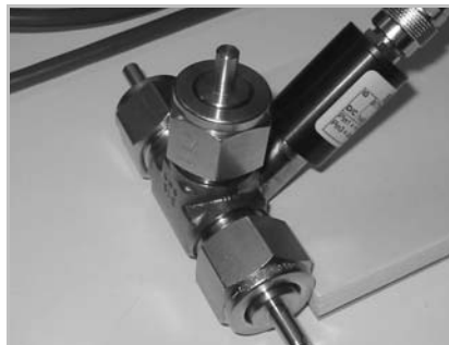
Figure 1: Swagelok based TPC Pressure Test Cell.
