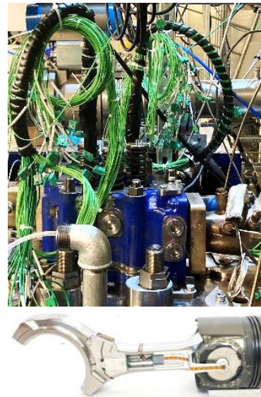
Figure 20: Thermal survey instrumentation
