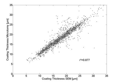
• Strong correlation of coating thickness data obtained from SEM and serial sectioning images (at the same position).
