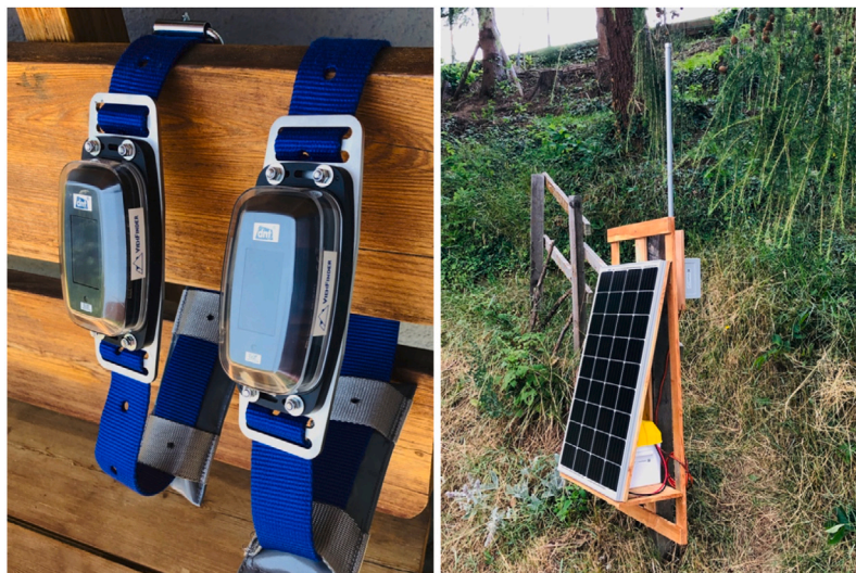
Fig. 1. The two major components of the ViehFinder setup. The ViehFinder collar for tracking the position (left) and the LoRaWAN antenna for data transmission to the server (right). Both are solar-powered.
