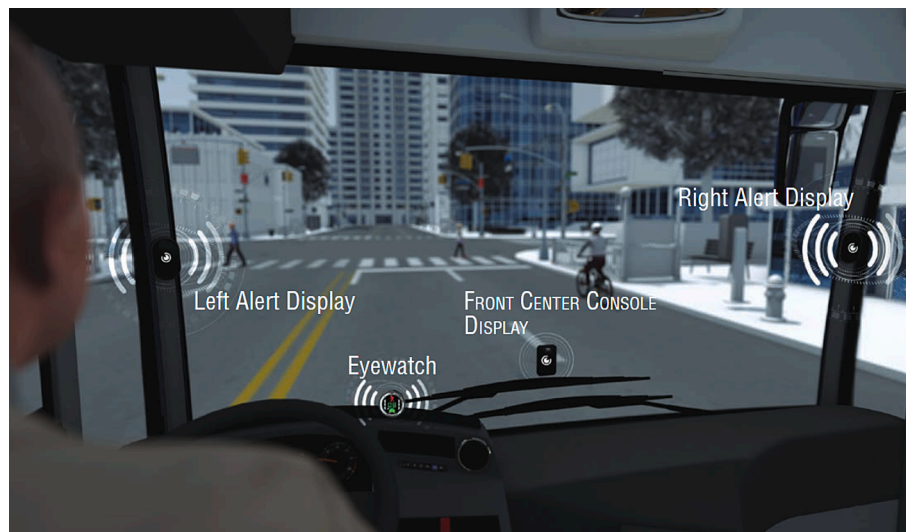
Fig. 2. Displays of the ME Shield+ (Mobileye Vision Technologies LTD, 2016b).
