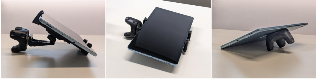
Fig. 3. A tablet with the tracker mounted to different positions. The tracker position in the far left image provides the best visibility for the base stations. The far right configuration adds the least weight to the handheld device. The middle image shows a compromise between the other two configurations.
