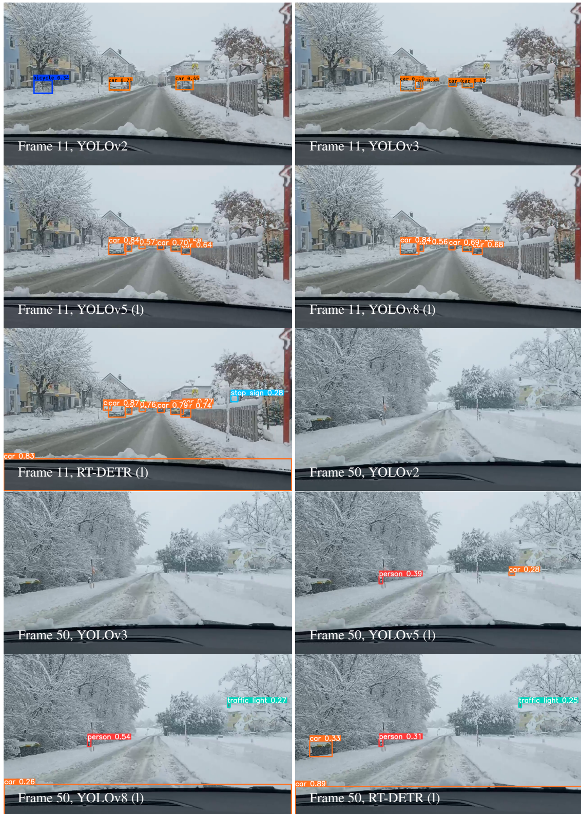
Figure 5: Deep learning vision object detection models applied to two example scene in AUT.
