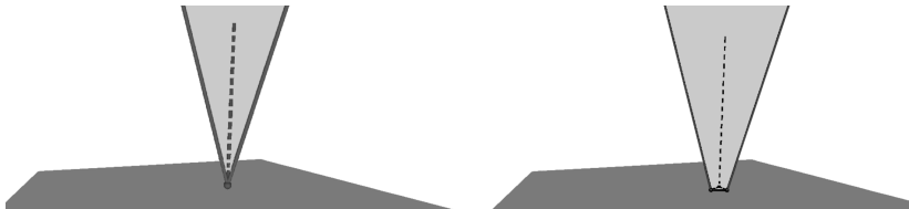
A degree-4 touching vertex and its offset surface
