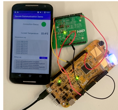
Fig. 4. Prototype showcasing the secure NFC BMS readout.
