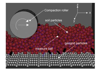
Figure 4. Generated model with the particle flow code.
