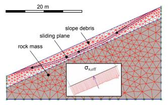
Figure 1. Example of a slope with geological known failure zone.
