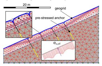
Figure 2. Slope with failure zone improved with geogrid and prestressed anchorage.
