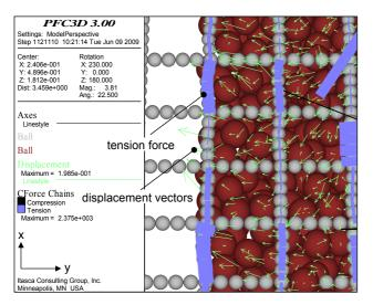
Figure 5. Qualitative trend of pre-stressing the reinforcement during compaction the soil-layer. The thickness of the blue line represents the tensile force in the geogrid string.
