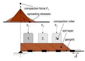
Figure 3. Schematic behavior of pre-stressing as a result of compaction.
