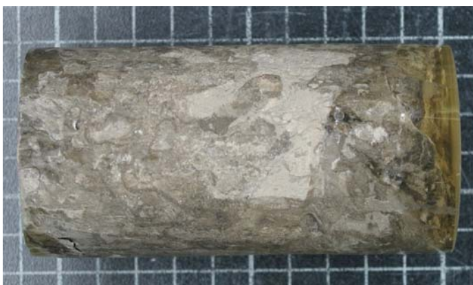
Figure 5. Specimen with resin reinforced end planes.
