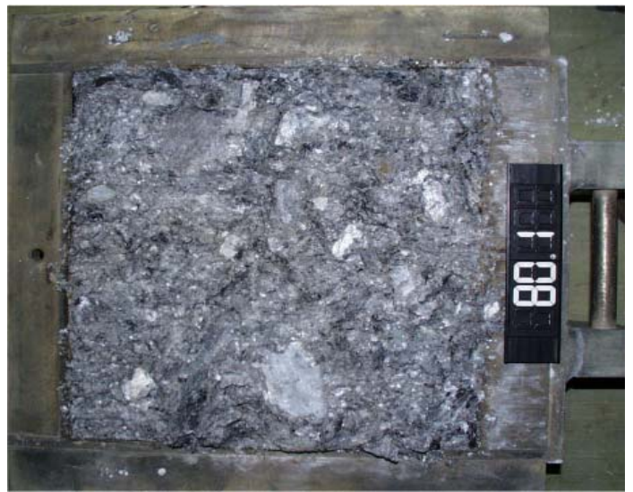
Figure 13. Picture of large-scale shear box test for remolded specimens (30 x 30 cm).
