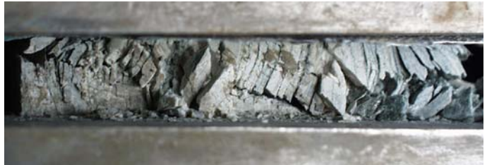
Figure 10. Deformations of intact phyllite tensile failures, interlayer shear and rigid block rotation.
