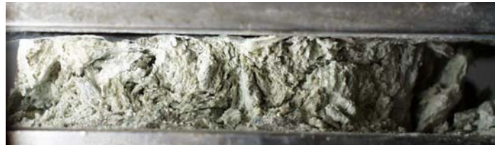
Figure 9. Deformations of weak faulted phyllite, brittle cataclastic flow – interlayer shear.
