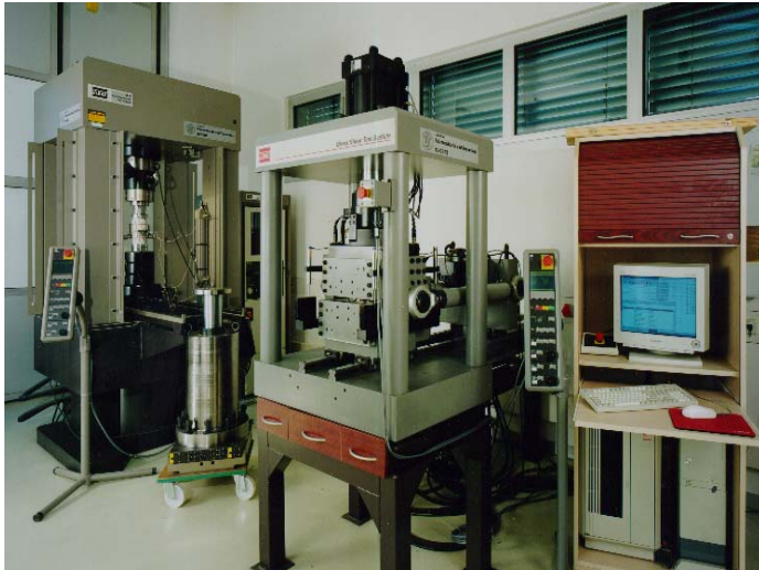
Figure 4. Equipment for a rock mechanics laboratory. Left: stiff load frame for UCS and triaxial tests. Centre: direct shear frame. Right: control unit.
