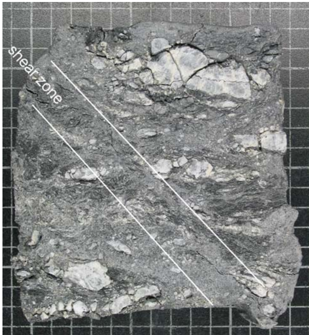
Figure 7. Sliced specimen after a triaxial test.
