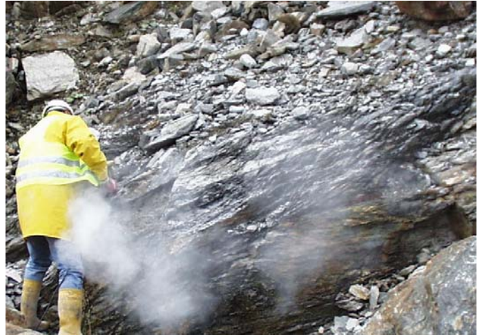
Figure 3. Sampling with manual work using a cutter.
