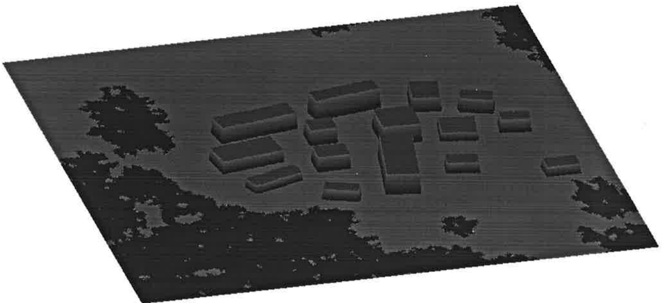
Figure 5. First site model with simple rectangular building blocks resulting from the combination of information from slant range shadows and interferometric height measurements. The area covers approximately 220 \times 220 \text{ m}^2 .
