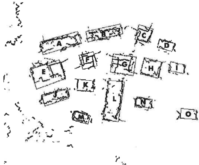
Figure 4. Reconstructed building walls of the whole building ensemble on the MOUT testsite with overlaid building outlines from ground truth data. The area covers approximately 180 \times 150 \text{ m}^2 .
