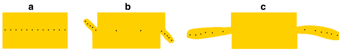
Fig. 13 Illustration of the evolution of the surface contaminants using point tracking. a Initial positioning of the points on the weld line. b Points are being extruded through the flash. c Contaminants completely removed
