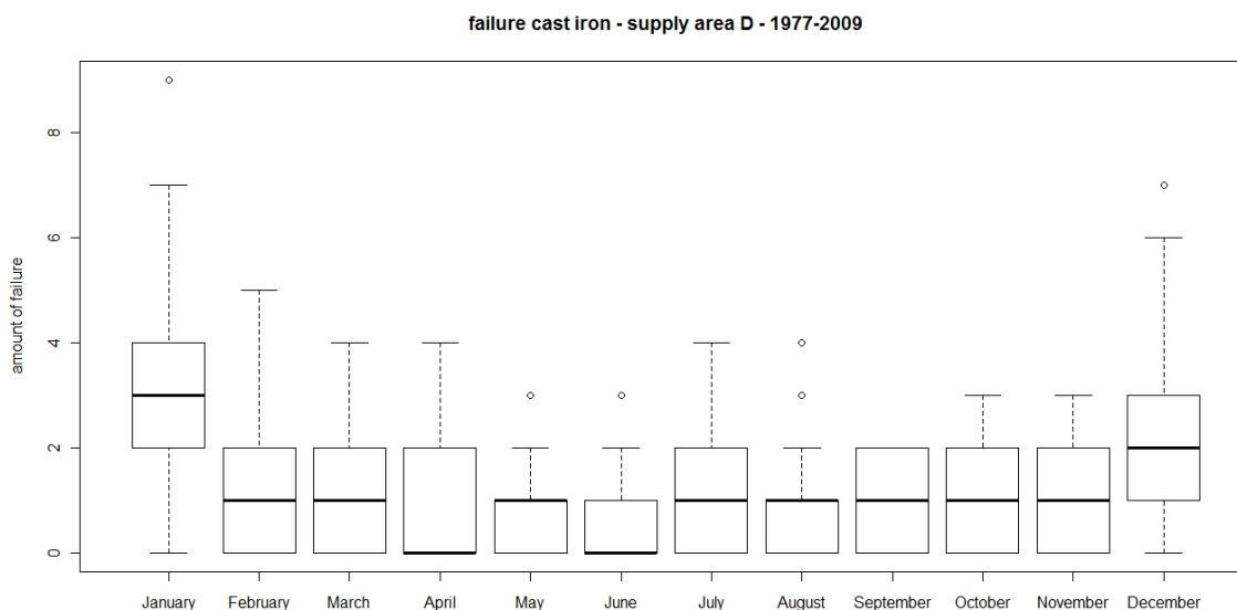
Figure 8: Variability of cast iron failure frequency for supply area D in the period 1977-2009
