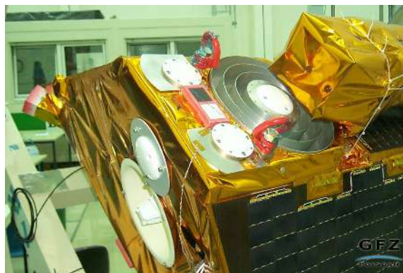
Figure 3.2: Rear section of the CHAMP satellite with three different GPS antennas. ©GFZ
