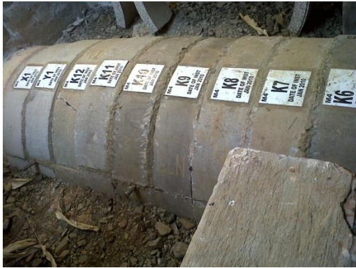
(a) Pipe sections (samples) of different concrete mixtures
