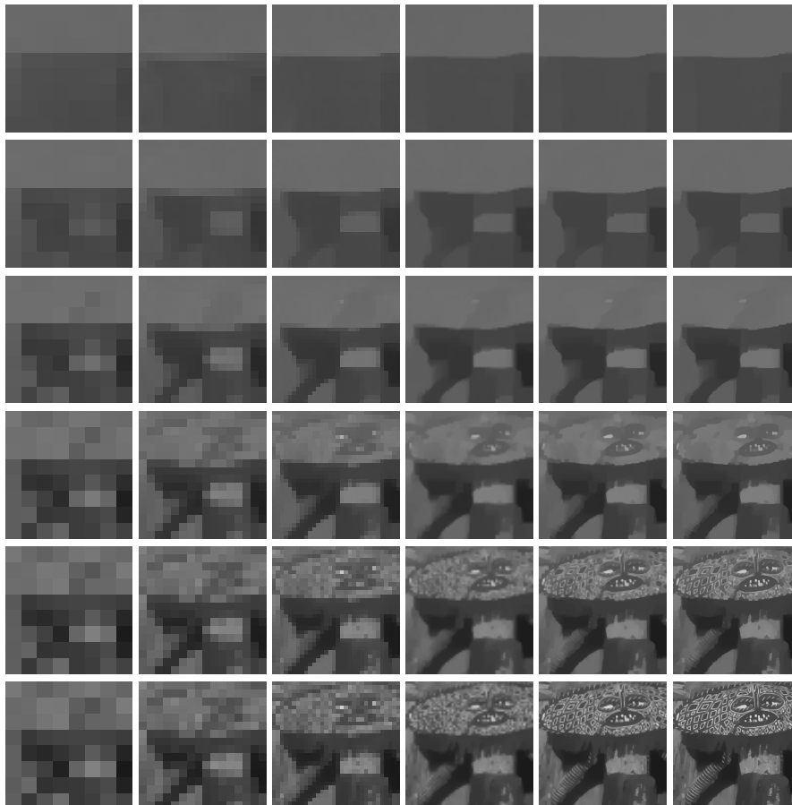
Fig. 1. Simple ROF model: Output of our network over 6 different resolution levels ( columns ) for 6 different smoothness costs ( rows ).
