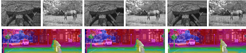
Fig. 4. Top: Denoising at 20% noise level. From left to right: Input; result; original. Bottom: Stereo examples from [32]. From left to right [9]; ours, trained via [9]; ours, trained via the truncated 3D distance function. Disparity color code: White - near, blue - far.
